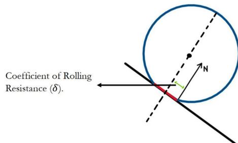
Figure 1. Defining the coefficient of rolling resistance
