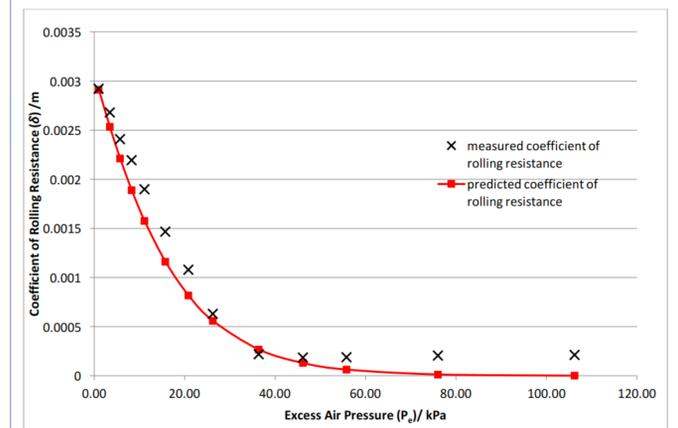
Figure 6. Measured values of coefficient of rolling resistance agrees with the values predicted using the Logistic function.
