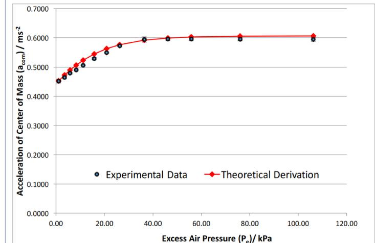
Figure 5. Logistic function gives a perfect fit for the experimental data which also Verifies the value of the maximum acceleration predicted to be  $0.61 \text{ ms}^{-2}$ .
