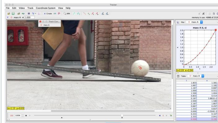
Figure 4. The measured acceleration was computed from the quadratic fit of the Position-time graph of the football using TRACKER.
